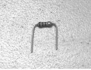
brown means "1", black means "0", yellow means "times 100  $\Omega$ "  $10~x~100~\Omega=1000~\Omega=1~\text{k}\Omega$
