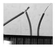
Insert the wires into a wire nut. Gently twist the wire nut clockwise until the connection feels snug.
