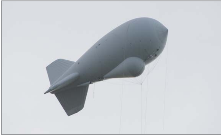
A 200-foot-long tethered aerostat blimp containing more than 2,000 pounds of radar gear, used by Customs and Border Protection at eight sites along the US/Mexico border. CLUI photo
