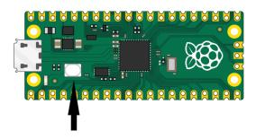
Press the BOOTSEL button and hold it while you connect the other end of the micro USB cable to your computer. A Raspberry Pi is shown in the image below, but the same applies to any computer.
